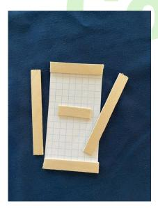
Step 5: Because the popsicle sticks are out of scale with the rest of the model, we will subtract the actual width of a stick's face from the top and bottom of our 8' flat (in scale) to get the measurement of our two **Stiles**. Do the same to get the measurement for one **Toggle**. Cut all three pieces and arrange them on one of the graph paper flat **Skin**.
