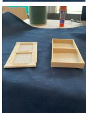
Next, we force the frame left or right so an adjacent **Stile** is flush to the Skin. Once we ensure the frame squared to that corner of the skin, we staple through the Skin into the Stile forming a perfectly square frame. Continue stapling around the flat across the Top Rail the remaining Stile.
