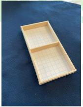
NOTE: When building a Hollywood flat in real life, we will do this same process of squaring the frame to the Lauan skin while the glue is still wet and BEFORE we fasten with staples. First we zig zag glue across all edges of the frame, then we set the Lauan skin on top.
