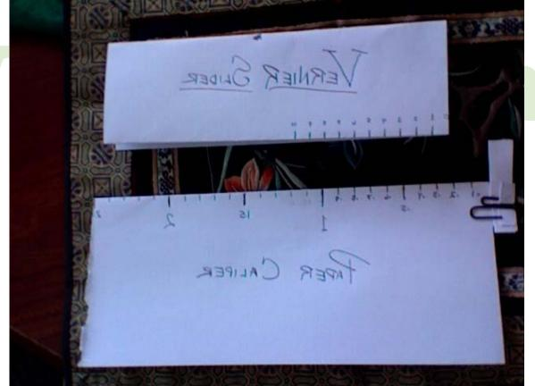
Now the students have made their own caliper and can try them out. They should mesure some object you supply ( pennies, length or pen, width of four fingers, etc.) In order to use the vernier scale the object cannot be much longer than 15cm.
