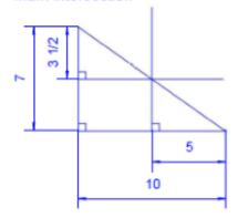
erect perpendicular on 90 degree side @ 1/3 legnth from 90 degree corner
